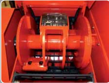
*The rotor with a diameter of 600 mm and 6 blades has a huge flywheel*
