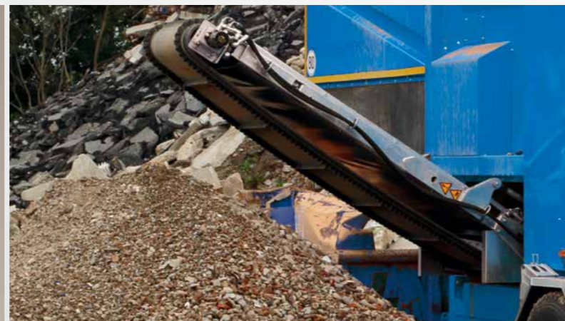
Discharge conveyor for heavy fraction
