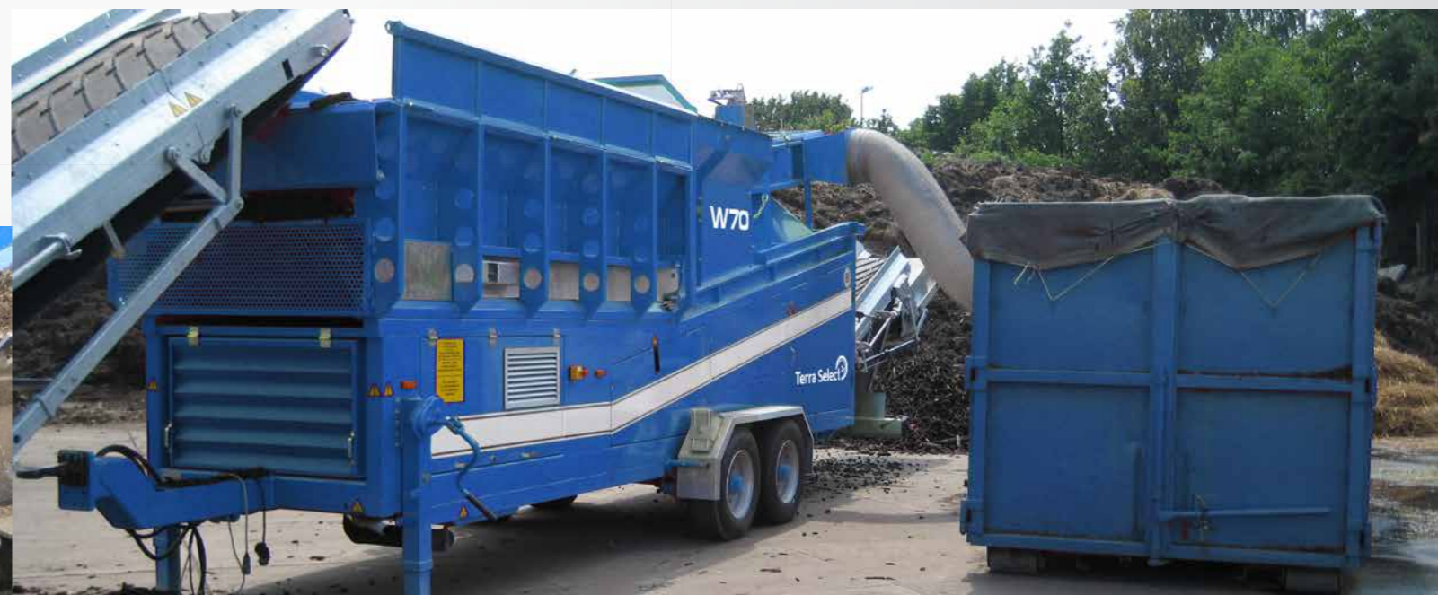
Windsifter - Terra Select W 70, optional feeding by wheel loader or directly by a screening machine.
