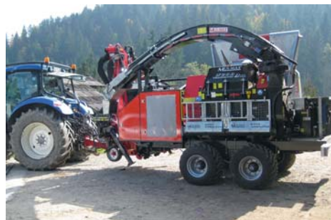
WT 9 XL DS on trailers with a 380 hp Mercedes diesel engine
