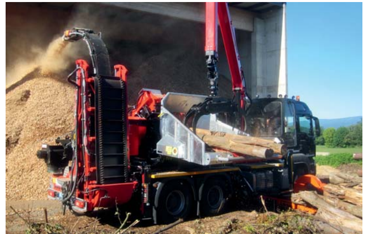
Wood chip discharge with blower
