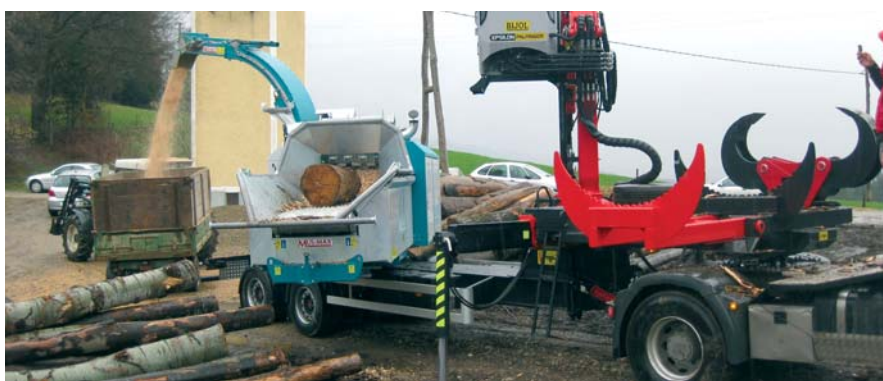
Hacker on saddle vehicle, can be swivelled left and right, with built-up wood splitter
