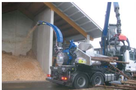
Hack-Truck with WT 7 L NMV Mercedes truck with 400 HP
