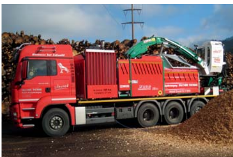
WT 10 XL on truck with diesel engine John Deere 600 HP, chopping machine with slewing ring and 3-m feed conveyor
