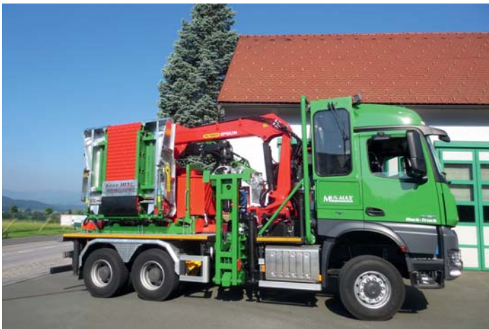
Hack Truck Mercedes WT 10 XL (520 hp) with NMV drive
