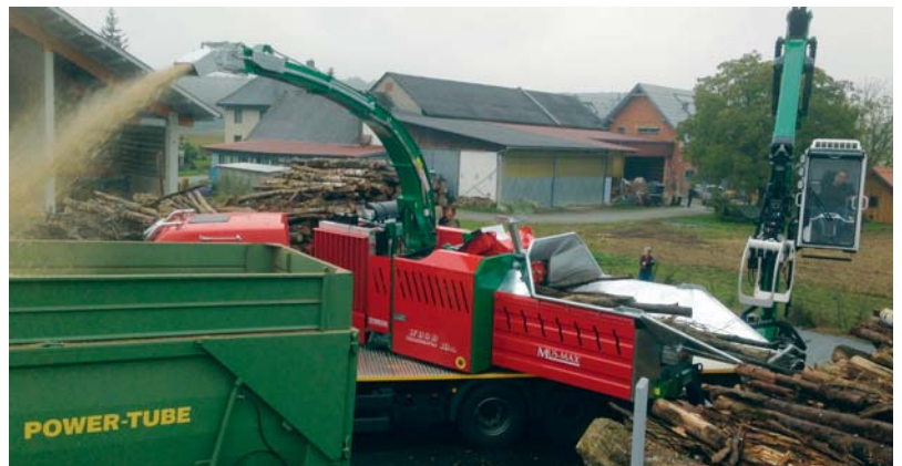
The lifting crane cab provides for excellent visibility at the chopping site.
