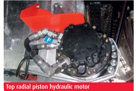
Top radial piston hydraulic motor
