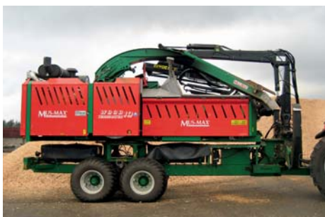
WT 10 XL DLK. WT 10 on underframe with diesel engine CAT C18 700 PS, chopping machine with slewing ring
