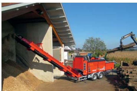
WT 10 XL DLB. Longitudinal machine CAT diesel engine 775 HP (conveyor belt discharge)
