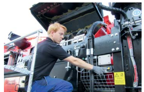
Top rotor cover – can be lifted hydraulically
