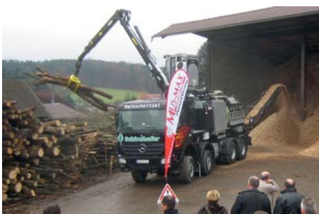
WT 11 DS set up on truck, with 500 HP diesel engine and discharge conveyor belt
