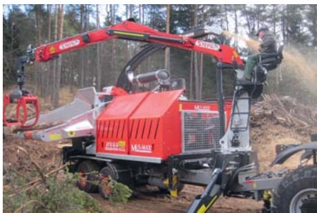
WT 8 XL with 245 HP John Deere engine on underframe
