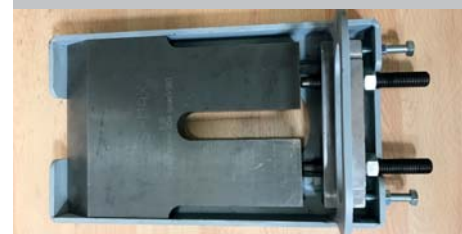
Top chopping knife setting gauge: quick blade change
