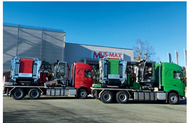
Hack Truck Volvo WT 10XL and WT 11 (up to 750 hp) with RBV intermediate gearbox
