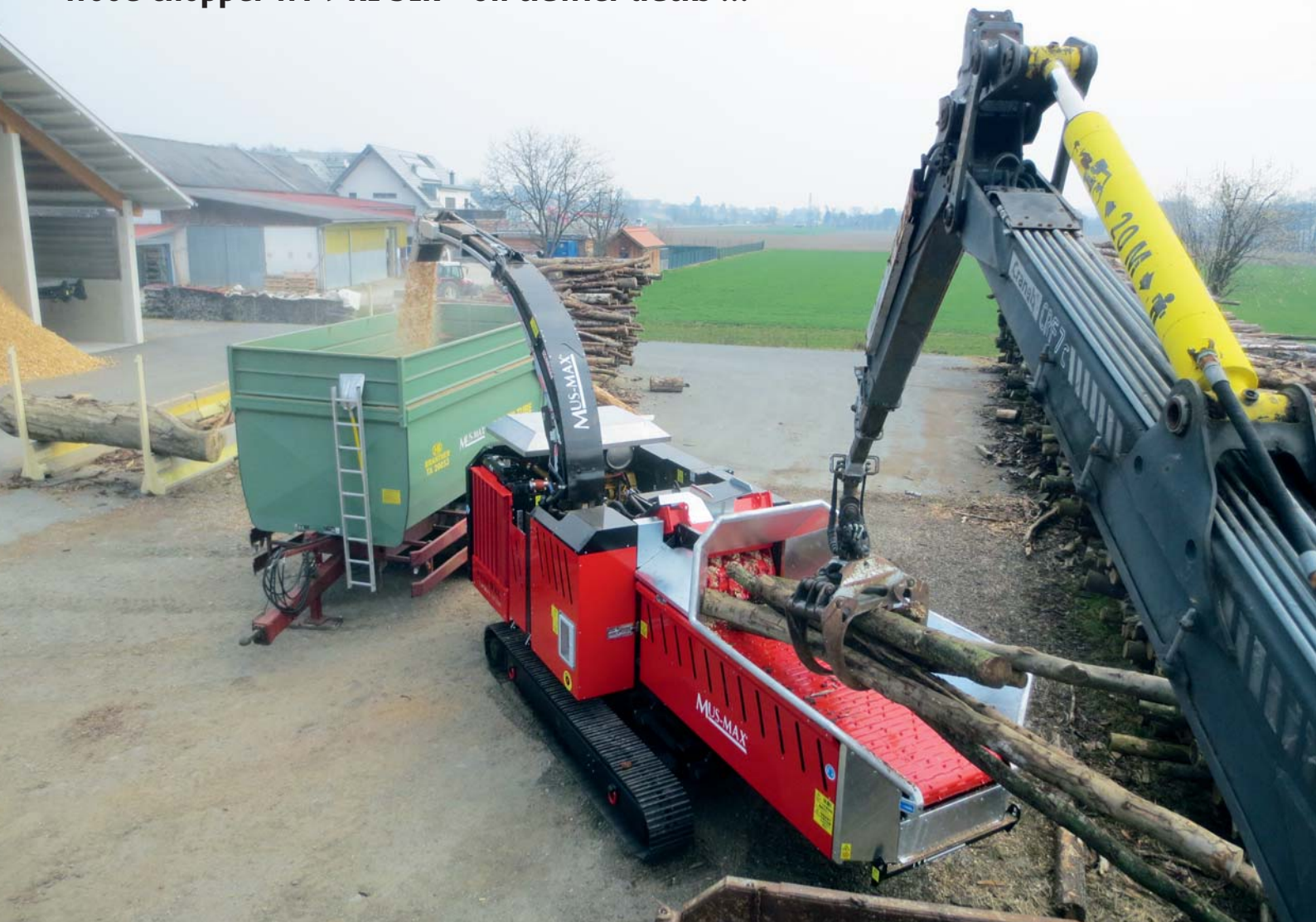
Wood Terminator 9 XL DLK wood chopper on a crawler chassis for Japan. Operation from the excavator by radio control.
