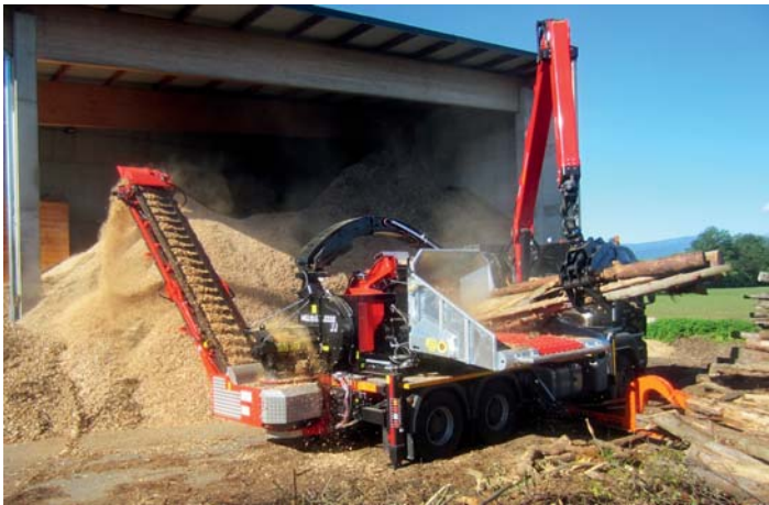
Wood chip discharge with conveyor belt
