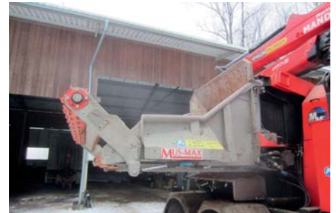
Top extension panel, hinged – feed length: 3.15 m
