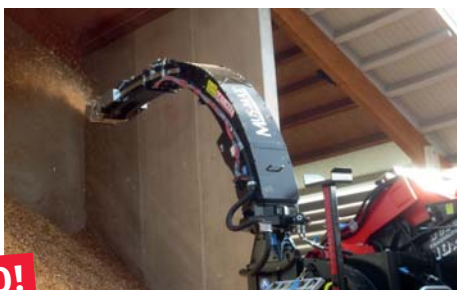
Blowing upwards with ejector is possible
