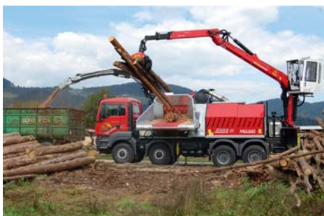
WT 11 on 4-axle truck MAN TGS 41/440 CAT diesel engine 775 HP
