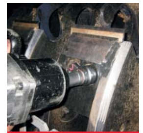
Blades quickly replaceable
