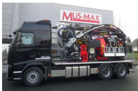
Hack truck WT 9 XL RBV with transmission from the main drive
