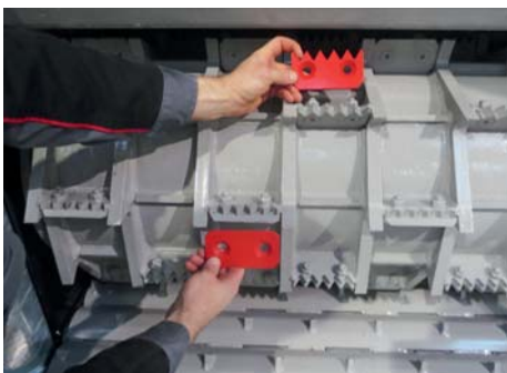
Crock System: Exchangeable knives and tines
