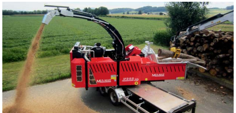
The chopper WT 10 XL DLK can also be set up on a trailer. This trailer has robust, hydraulic support feet. The chopping vehicle can be towed with a tractor or a truck.
