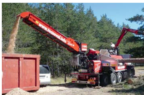
WT 9 XL DS with ascending screw and conveyor belt on MAN truck, driven by 450 HP John-Deere diesel engine
