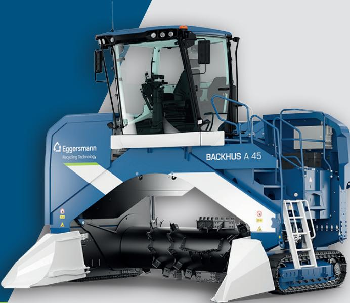
The BACKHUS A 45 marks the beginning of our midsize range – yet it shines as a true powerhouse in a market comparison: with a windrow width of up to 4.5 m and a maximum windrow height of 2.3 m, it achieves a turning capacity up to 3,000 m<sup>3</sup> per hour, depending on the material.
